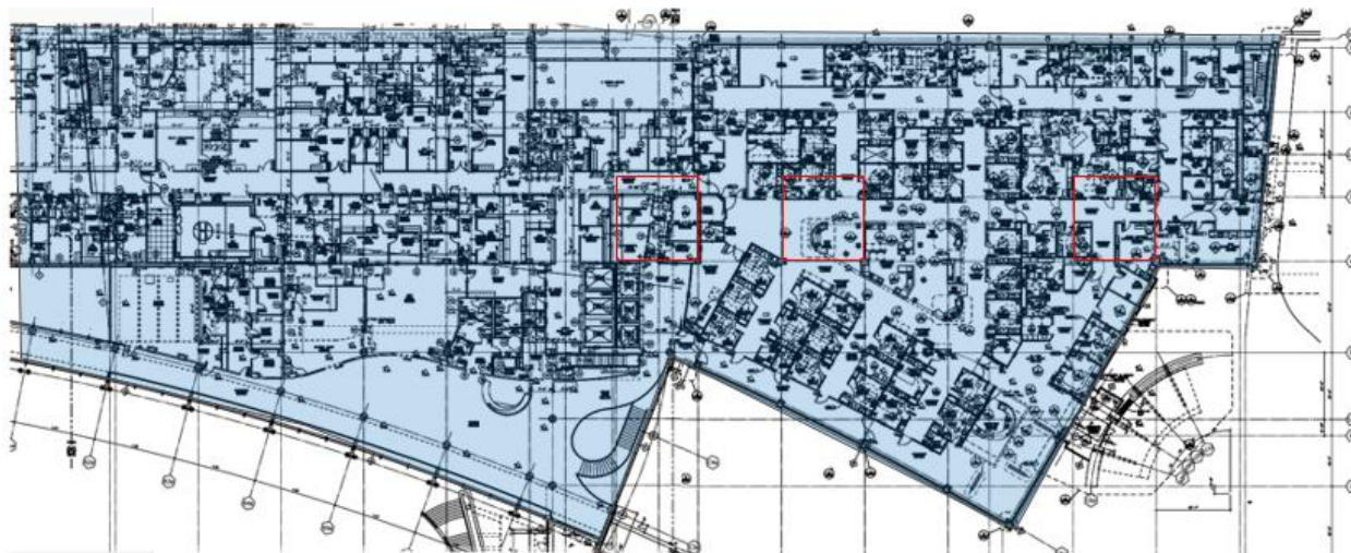
Figure 6: Architectural Plan of Bed Tower (example typical 30'x30' bays in red)
