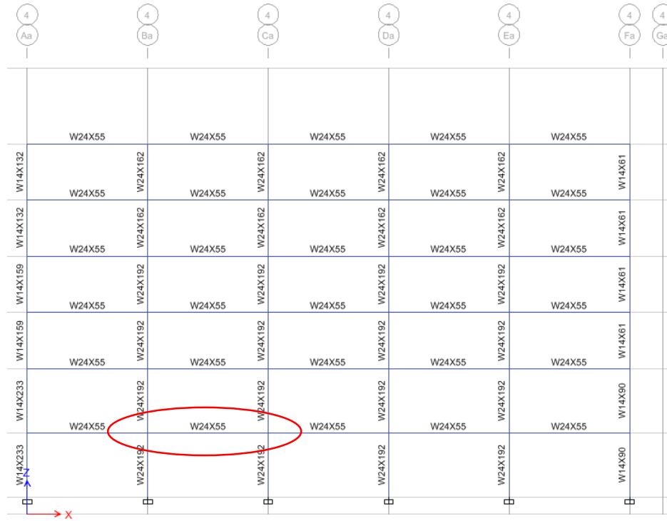
Figure 17: Special Moment Frame Section Assignments
